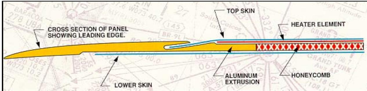
The NOFOD® Heater Panel becomes a structural part of the wing.
